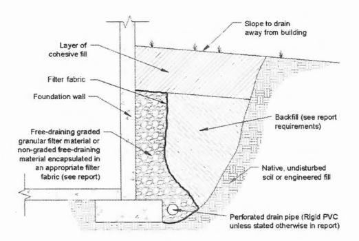
As an alternative to free-draining granular fill, a pre-fabricated drainage composite may be used. A pre-fabricated drainage composite is a plastic drainage core or mesh which is covered with filter fabric to resist soil intrusion, and fastened to the wall prior to placing backfill.
