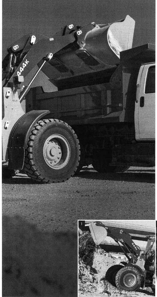
Powerllel's unique design separates the bell crank from the cross tube, attaching instead to the loader frame via a Y-shaped link. This "freefloating" bell-crank design allows load forces to work with, not against, the boom. For powerful breakout in tough digging.
