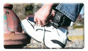
Figure 44. Field Replaceable Battery and Strap
