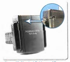
Figure 27. Physical Evidence of Tamper
