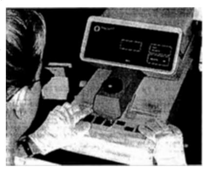
Two uniform density targets are filmed at the beginning and end of each roll. The uniform density target can be as simple as a blank sheet of white bond paper, but **it must be as large as, or larger than, the materials being filmed**.
