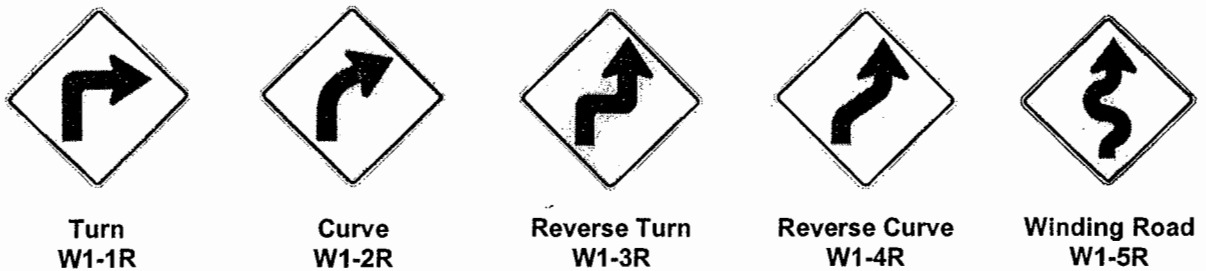
Figure 5. Curve and Turn Signs
