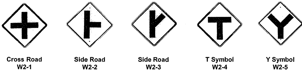
Figure 3. Intersection Warning Signs
